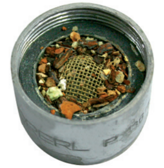
Rust particles in a tap sieve indicate corrosion is present
