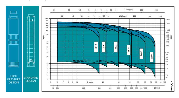
Z6 series operating characteristics at 60 hz.
